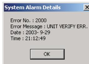
The dates and times of the PLC CPU stopping errors and PLC CPU errors displayed in the system alarm details dialog box are those when the errors occurred in the CPU module (dates and times according to the internal clock of the CPU module).
