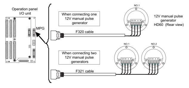
(Note 1) When selecting a manual pulse generator, make sure that its case and 0V terminal are insulated.(Note 2) Select 25pulse/rev or 100pulse/rev on the parameter screen.
