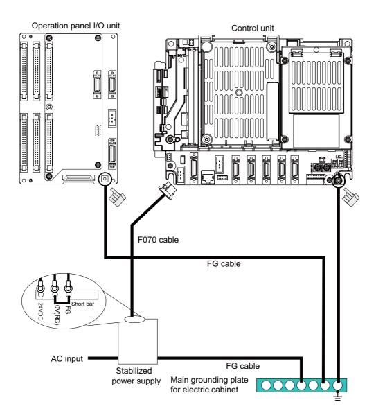
(Note) "24VDC" represents (+) side (24VDC) of 24V stabilized power supply, while "0V(RG)" represents (-) side. "FG" (Frame Ground) corresponds to the general expression "PE" (Protective Earth).
