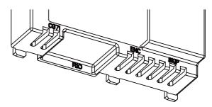
$\ensuremath{\left(2\right)}$  Insert two snap-fits on the top right and left edges of the cover into the control unit.
