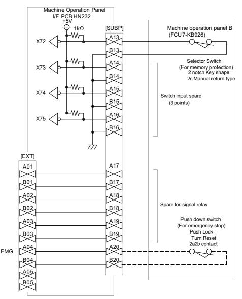
(Note1) Wirings for selector switches must be directly soldered to terminals or use tab terminals (110 series).
