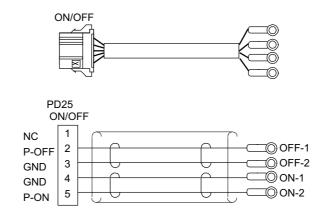
[ON/OFF] Connector: 1-178288-5 Contact: 1-175218-5 Recommended manufacturer: Tyco Electronics
