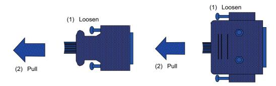
Do not connect or disconnect the cables between units while the power is ON.
