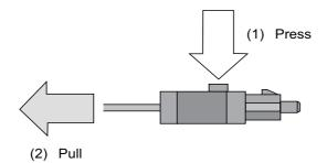
(f) For the Ethernet connector, pull off while holding down the locked latch.
