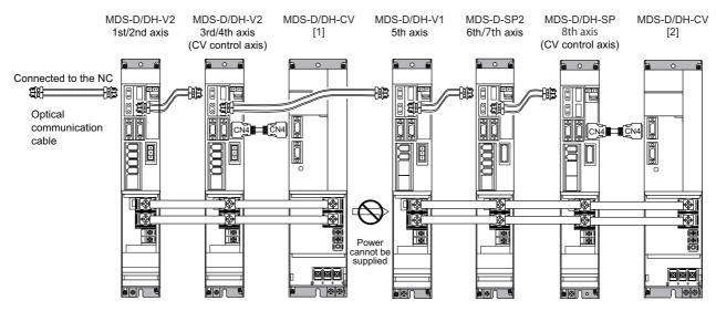
Connections when using two or more power supply units within a single NC communication bus system
