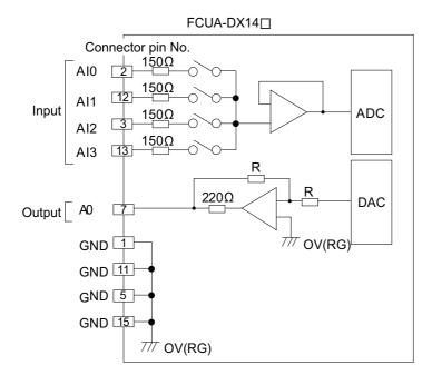
Connect the cable to the designated connector. Incorrect connections could damage the device.
