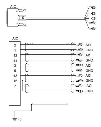
[AIO] Connector: 10120-3000VE Case: 10320-52F0-008 Recommended manufacturer: 3M Wire material: UL1061-2464 AWG24 × 6P Recommended manufacturer: Oki Electric Cable
