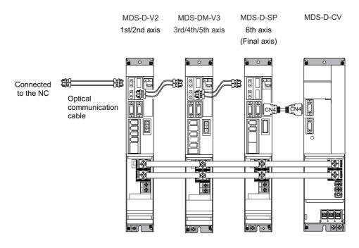
The optical communication cables from the NC to the final drive unit must be within 30m.
