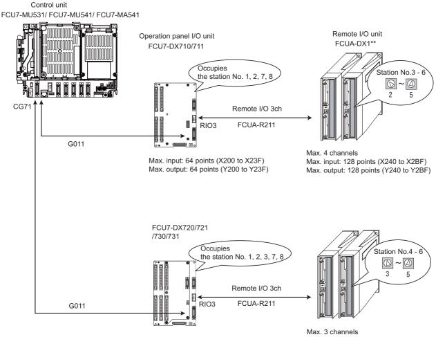
Max. input: 96 points (X200 to X25F) Max. output: 96 points (Y200 to Y25F) Max. 3 channels Max. input: 96 points (X260 to X2BF) Max. output: 96 points (Y260 to Y2BF)
