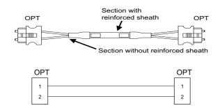
[OPT] Connector: PF-2D103 Recommended manufacturer: Japan Aviation Electronics
