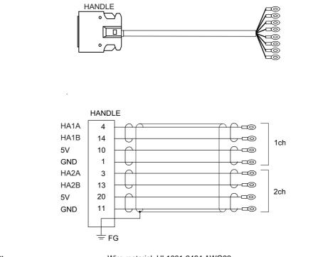
[HANDLE] Connector: 10120-3000VE Case: 10320-52F0-008 Recommended manufacturer: 3M Wire material: UL1061-2464 AWG22 × 6P Recommended manufacturer: Oki Electric Cable
