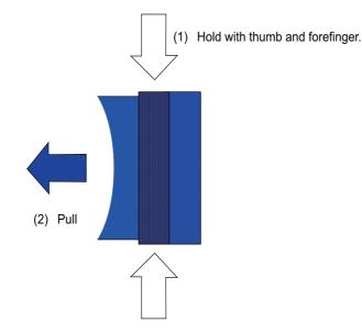
(d) For the screw fixed type connector, loosen the two fixing screws, and pull the connector off.
