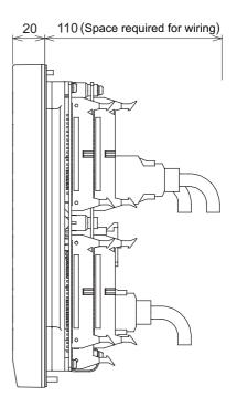
(Note) The above side view shows the state with the operation panel I/O unit FCU7-DX720/DX721 mounted.
