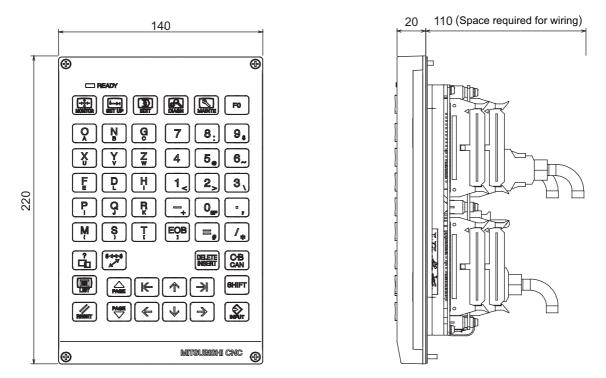
(Note) The above side view shows the state with the operation panel I/O unit FCU7-DX720/DX721 mounted.
