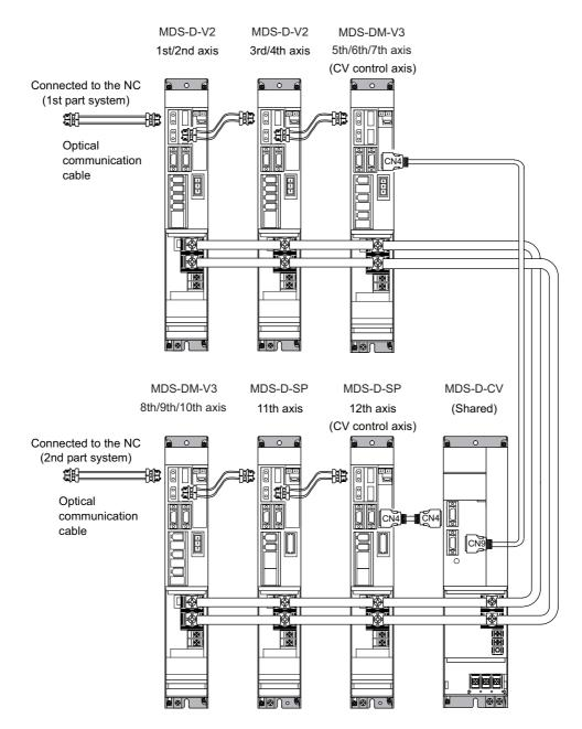
Connections when using one power supply shared by two NC communication bus systems
