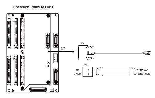
The analog signal output circuit can be used only for the FCU7-DX720/DX721.
