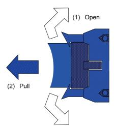
(c) For a flat cable type connector without latches, hold the connector with a thumb and forefinger, and pull the connector off.
