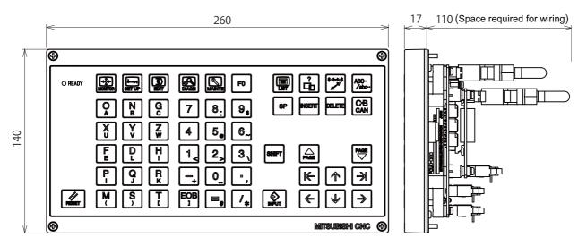
(Note) The above side view shows the state with the operation panel I/O unit FCU7-DX720/DX721 mounted.
