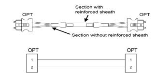
[OPT] Connector: CF-2D101-S Recommended manufacturer: Japan Aviation Electronics Wire material: Hard clad type PCF optic cable Recommended manufacturer: Oki Electric Cable
