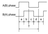
a.b.c.d.e: A phase or B phase rising edge (falling edge) phase difference =  $T/4 \pm T/10$ T: A or B phase cycle
