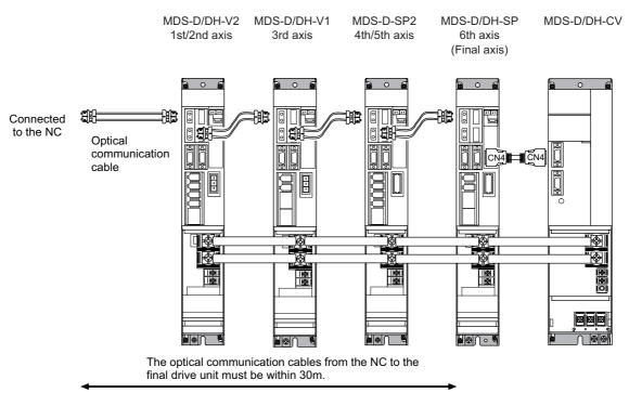
Connection when using one power supply unit
