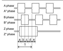
a.b.c.d.e: A phase or B phase rising edge (falling edge) phase difference =  $T/4 \pm T/10$
