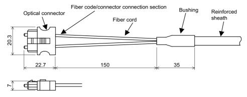
To ensure the system performance and reliability, purchase the optical communication cable from Mitsubishi. A machining drawing is given in "Cable" as reference, but the purchased optical communication cable cannot be cut or connected by the machine tool builder.
