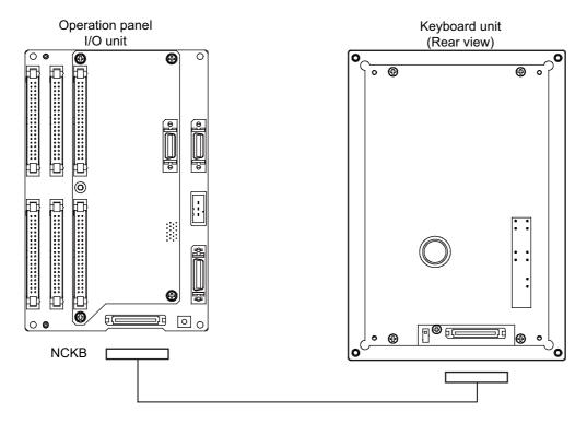
(Note) Firmly insert the connection cable until it is locked.
