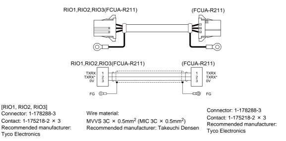
(Note) Fold the cable shield over the sheath, and wrap copper foil tape over it. Connect the wound copper foil tape to GND plate of the connector.
