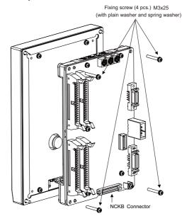
(Note) Use M3x25 screws (with spring washer and plain washer) when mounting the operation panel I/O unit.
