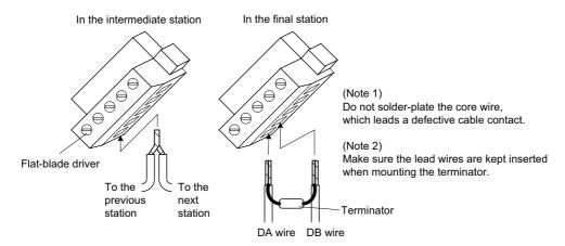
(6) After wiring cables to the terminal block, Mount the terminal block into the CC-Link connector and fix it with a flat-blade screwdriver.
