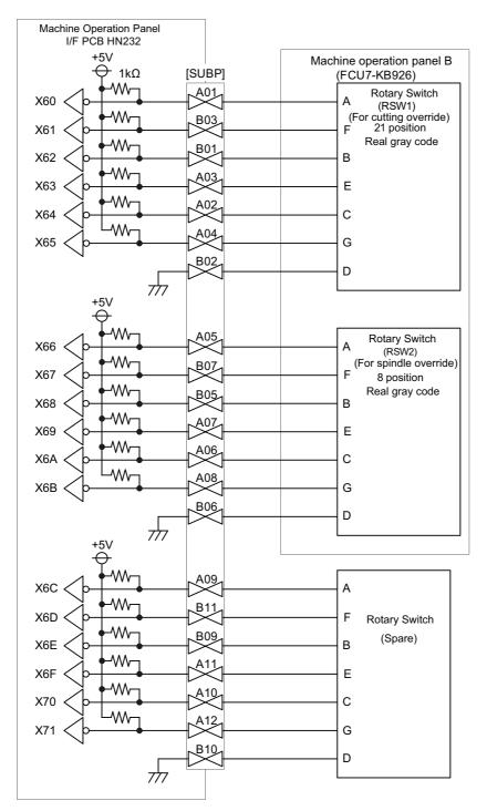
(Note1) Use the special lead wire with a connector for wiring of rotary switch.
