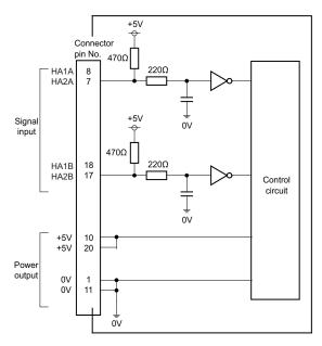
When using the synchronous feed encoder and the manual pulse generator at the same time, connect the manual pulse generator to the operation panel I/O unit or use a distribution cable made by the machine tool builder.
