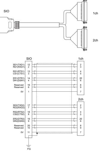
[SIO] Connector: 10120-3000VE Case: 10320-52F0-008 Recommended manufacturer: 3M Wire material: UL1061-2464 AWG24 × 12P Recommended manufacturer: Oki Electric Cable [1ch][2ch] Connector: CDB-25S Contact: CD-SC-111 × 9 Lock nut: HD-LNA × 2 Recommended manufacturer: Hirose Electric
