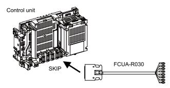
(Note) Connecting the skip signal cable to a wrong connector causes a damage on the control unit when turning ON the skip signal power supply. Confirm the wiring before turning the power ON.
