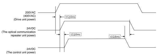
t1: Time lag between the power-ON of the drive unit and the optical communication repeater unit
