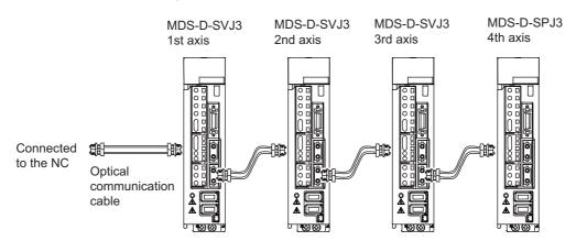
The optical communication cable up to 5m can be used in G396 series, and up to 20m in G380 series.
