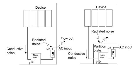
(Note 1) The conductive noise can be suppressed by inserting a noise filter, but the radiated noise will flow out.(Note 2) The conductive and radiated noise can both be suppressed by adding a partition plate to the noise filter.
