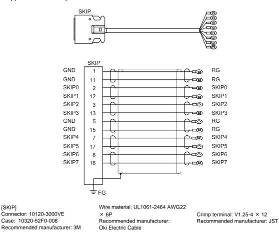
(Note) Fold the cable shield over the sheath, and wrap copper foil tape over it. Connect the wound copper foil tape to GND plate of the connector.
