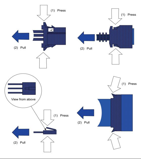
Do not connect or disconnect the cables between units while the power is ON.
