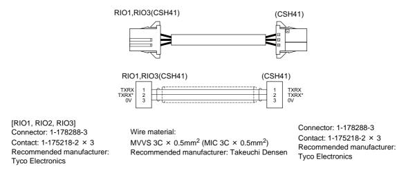
(Note 1) Protect both ends of the cable with insulated bushing.
