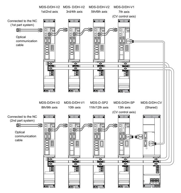
Connections when using one power supply shared by two NC communication bus systems
