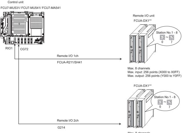
Max. 8 channels Max. input: 256 points (X100 to X1FF) Max. output: 256 points (Y100 to Y1FF)
