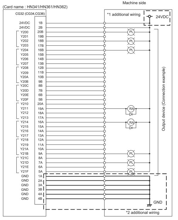
(Note 1) Connect +24V to either or both of the flat connector 1B, 2B (24VDC). (\*1)
