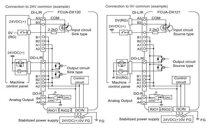
1. Connect the cable to the designated connector. Incorrect connections could damage the device.
