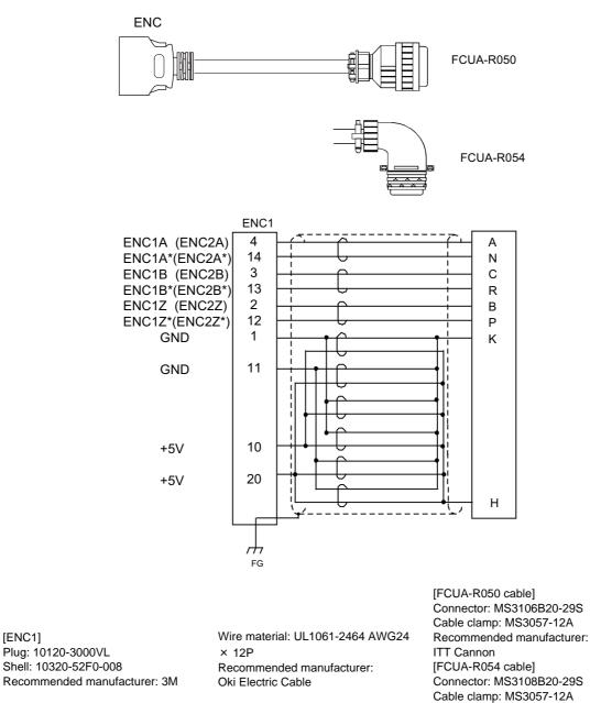
(Note) Fold the cable shield over the sheath, and wrap copper foil tape over it. Connect the wound copper foil tape to GND plate of the connector.
