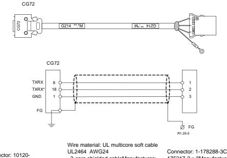
[CG72]Connector: 10120-3000VECase: 10320-52F0-008Manufacturer: Tyco Electronics UL2464 AWG24 3-core shielded cableManufacturer: Shinko Electric Wire Co., Ltd (If this cable is unavailable, find an equivalent one.) Connector: 1-178288-3Case: 1-175217-2 x 3Manufacturer: Tyco Electronics Crimp terminal: R1.25-5
