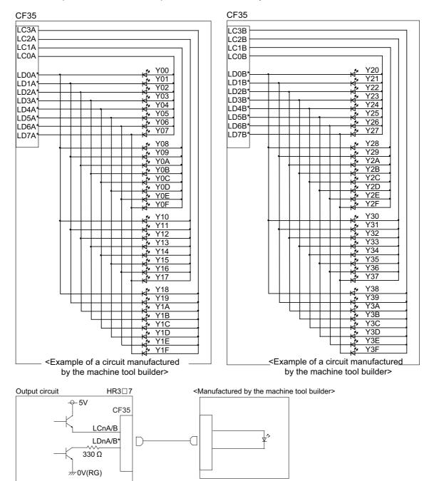
The common signals are changed over with scan output as shown in the following drawing. The LED outputs data, and lights only when the common signal is HIGH. The common signal changes to 4 signals in succession, and light s once every 5.84ms for 1.46ms only. The scan output is a 5V system.
