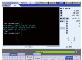
When the graphic drawing is completed, "Program check completed" message is displayed and the graphic drawing mode will be canceled.
