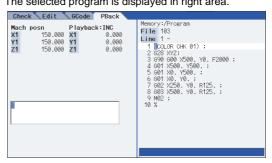
(Note 1) When the program is not displayed in the right area, a playback editing will not be executed. (Note 2) When the incremental value is set, playback movement amount will be cleared to 0 for all axes.
