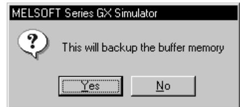
Click on the  Yes button, to save the entire device memory or the buffer memory for the slots allocated to special function modules in the I/O assignment settings.
