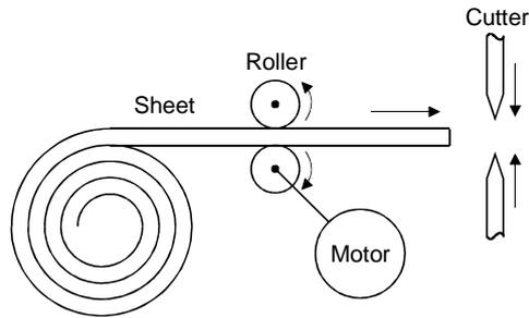
2) Turning X2 ON (Sheet feeding complete → Start cutting)
