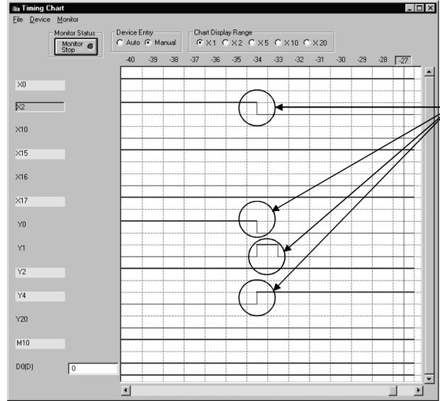
When X2 is turned OFF, Y0 is turned OFF, Y1 is turned ON for one scan and Y4 is turned ON.
