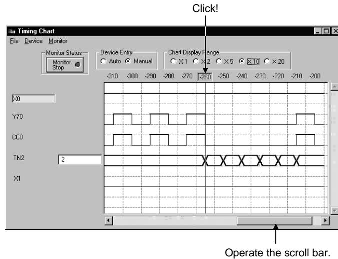
(c) By clicking "-260", the device status of 260 scans before will appear in \*1. In \*1, the bit device ON/OFF status and word device value are displayed.
