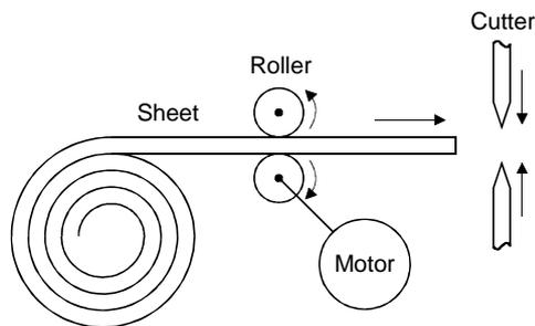
4) Turning X2 ON (Sheet feeding complete → start cutting)
