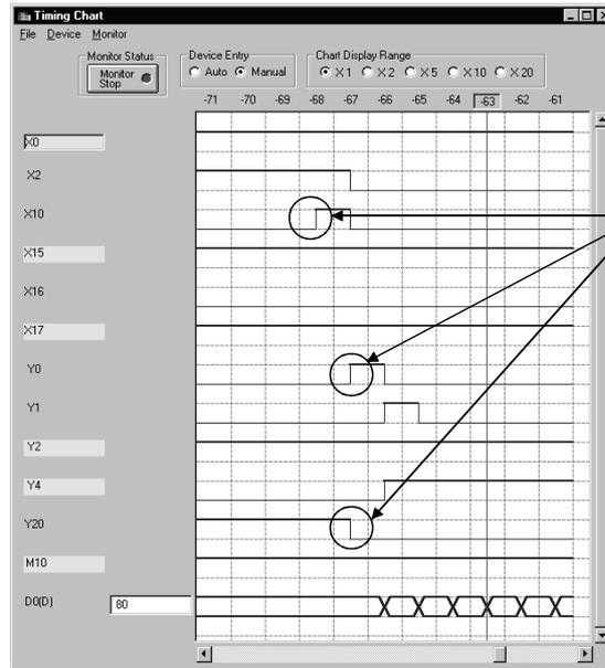
Turning on X10, turns on Y0 and turns off Y20.
