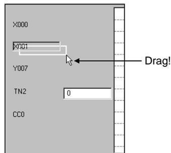
(b) By superimposing white square frame on the device name to be exchanged, device name can be exchanged.
