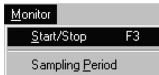
3) Device displayed on GX Developer screen will automatically be registered as device, and monitoring will start. (Maximum 64 devices can be entered.)
