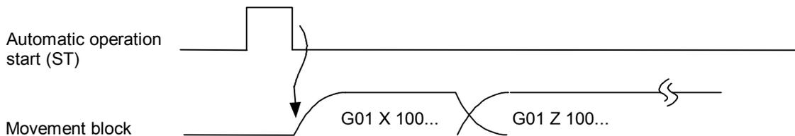
Automatic operation startup is performed on a part system by part system basis.
