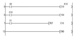
(2) The following program sets the value for C10 at 10 when X0 goes ON, and at 20 when X1 goes ON.
