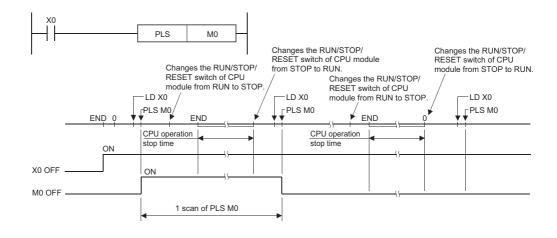
(3) When designating a latch relay (L) for the execution command and turning the power supply OFF to ON with the latch relay ON, the execution command turns OFF to ON at the first scan, executing the PLS instruction and turning ON the designated device.
