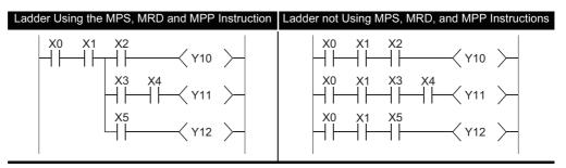
2. The number of times the MPS and MPP instructions are used must be the same
