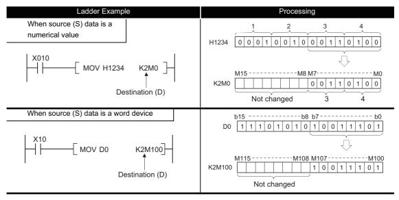
Fig 3.3 Ladder Example and Processing Conducted
