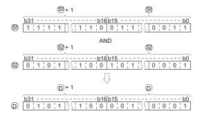
(2) For bit devices, the bit devices below the points designated by digit specification are regarded as "0" in the operation. (See Program Example (3))
