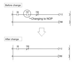
(2) Contact closed ....... LD, LDI changed to NOP (Note carefully that changing the LD and LDI instructions to NOP completely changes the nature of the ladder.)
