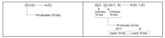
Fig. 2.2 Type of Processing Performed by Individual Instructions
