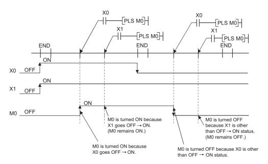
When specifying output (Y) in PLS instructions, the ON/OFF status of the device at the execution of the last PLS instruction in the scan is returned as the output (Y).
