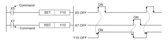
(3) When the execution command is OFF, the status of devices does not change.
