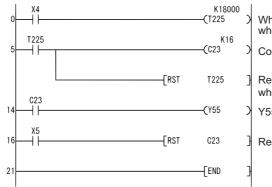
When T225 is set as retentive timer, it is turned ON when X4 ON time reaches 30 min.
