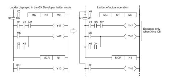
Inputting contacts on the vertical bus is not necessary when programming in the write mode of the GX Developer.
