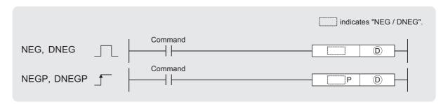
① : Start number of the devices where the data for which complement of 2 is performed is stored (BIN 16/32 bits)
