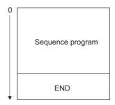
(2) END instruction is automatically set by the GX Developer during programming.
