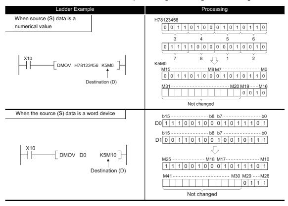
Fig 3.6 Ladder Example and Processing Conducted
