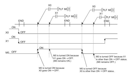
When specifying output (Y) in PLF instructions, the ON/OFF status of the device at the execution of the last PLF instruction in the scan is returned as the output (Y).
