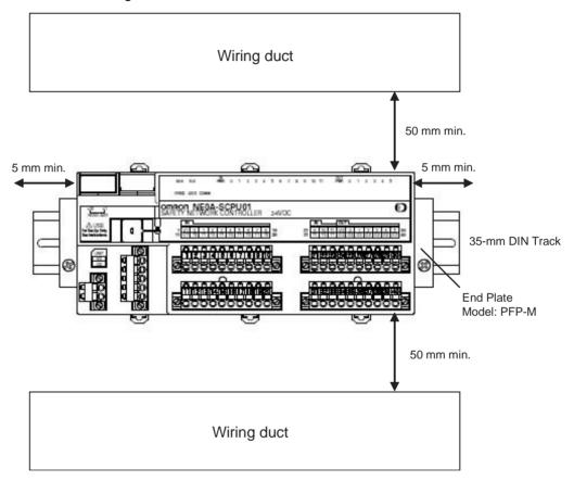
**Note** The NE0A-series Controller can be mounted only to DIN Track. Do not screw the Controller to the control panel.
