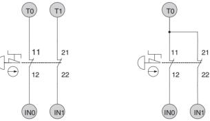
Circuit in Which Short Circuit Detection C between Input Signals Is Required. b
