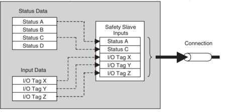
Sample 1: Transmitting both Status Data and I/O Tags as Safety Slave Inputs
