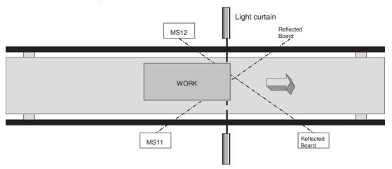
MS11: Muting sensor connected to Muting Signal 11 MS12: Muting sensor connected to Muting Signal 12
