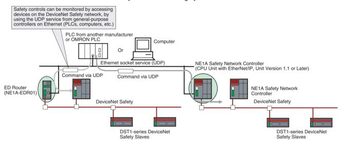
**Note** Refer to the *EtherNet/IP-DeviceNet Router Operation Manual* (Cat. No. Z912) for details on the NE1A-EDR01 EtherNet/IP-DeviceNet Router.
