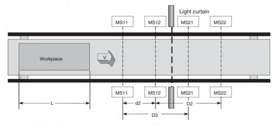
MS11: Muting sensor connected to Muting Signal 11 MS12: Muting sensor connected to Muting Signal 12 MS21: Muting sensor connected to Muting Signal 21 MS22: Muting sensor connected to Muting Signal 22
