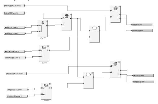
Local Input and Test Output Setting Example
