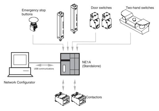
**IMPORTANT** Use a USB port connection to disable the DeviceNet communications (standalone). With Controllers that support EtherNet/IP, either the USB port or EtherNet/IP can be used. DeviceNet communications are stopped after DeviceNet communications are disabled (standalone), so the setting cannot be made from the DeviceNet port.
