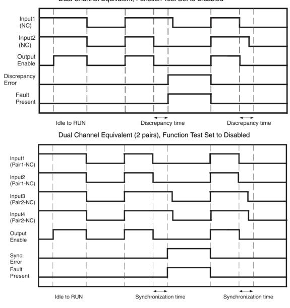
Dual Channel Equivalent, Function Test Set to Disabled
