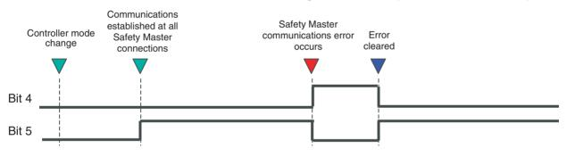
• Example: Monitoring NE1A-series Controller Safety I/O Communications Error and Status Flags from the PLC (when d5 and d6 Errors Occur)
