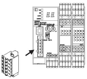
Stickers are placed on the communication connectors based on the color of each communications wire. By matching the communications wire colors with the connector sticker colors, you can check to see if wires are in the correct locations. The colors of the wires are as follows:
