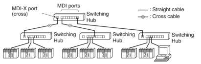
• Some switching hubs can automatically distinguish between MDI and MDI-X. When this kind of switching hub is being used, straight cable can be used between switching hubs.
