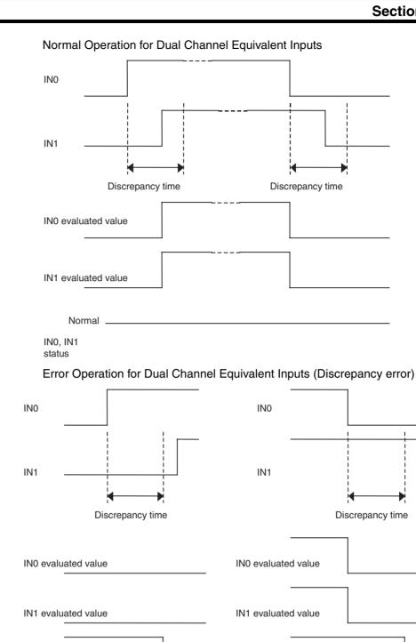
Note The NE1A-series Controllers supports function blocks with functionality equivalent to Dual Channel Mode. If Dual Channel Mode is set in a function block, then the safety input terminal can be set to Single Channel Mode.
