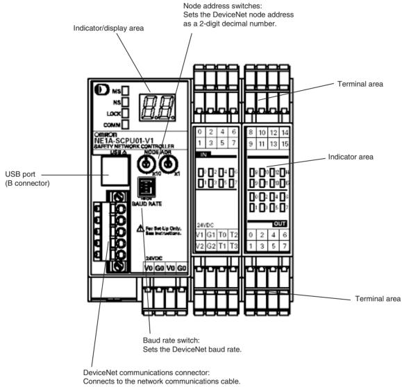
The power for communications is also supplied from this connector. The XW4G-05C1-H1-D Connector is provided for node connections.
