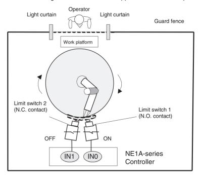
**Note** In the above example, limit switch 1 is wired to IN0 on the NE1A-series Controller and limit switch 2 is wired to IN1. Set the dual channel mode for local input in the NE1A-series Controller to dual channel complementary.
