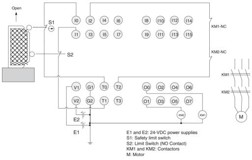
**Note** Connect a 24-VDC power supply to terminals V0 and G0 (power supply terminals for internal circuits).
