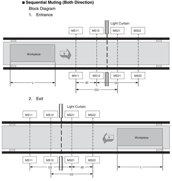
MS11: Muting sensor connected to Muting Signal 11 MS12: Muting sensor connected to Muting Signal 12 MS21: Muting sensor connected to Muting Signal 21 MS22: Muting sensor connected to Muting Signal 22
