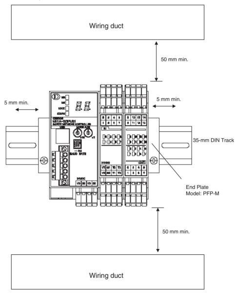
**Note** The NE1A-series Controller can be mounted only to DIN Track. Do not screw the Controller to the control panel.
