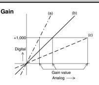
Gain determines the angle or slope of the calibration line, identified at a digital value of 1000.
