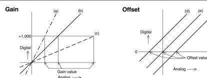
Gain determines the angle or slope of the calibration line, identified at a digital value of 1000.
