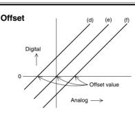
Offset is the 'Position' of the calibrated line, identified at a digital value of 0.
