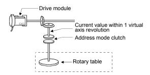
Current value within 1 virtual axis revolution = (Drive module travel value  $\times$  gear) %ND (% : Remainder operator) PLS 0 0 0 0
