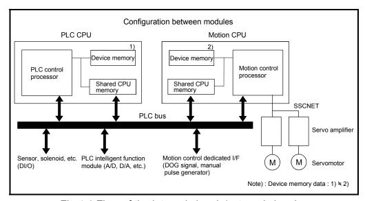
Fig.4.1 Flow of the internal signals/external signals
