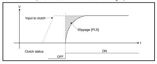
b) Since the slippage remains constant even if the drive module speed changes, the clutch ON/OFF position can be controlled without any influence from speed changes.
