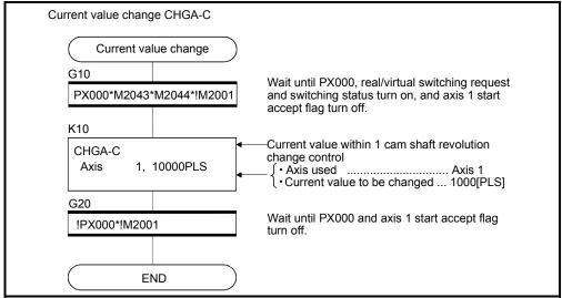
(Note): Example of the above Motion SFC program is started using the automatic start or PLC program.
