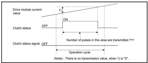
(f) When the mode setting device becomes "3", the clutch ON/OFF control starts based on the setting data while the clutch ON/OFF command device is ON.
