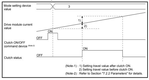
(g) When the mode setting device becomes "3", the clutch status turns OFF, while the clutch ON/OFF command device is OFF and the clutch status is ON.
