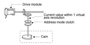
Current value within 1 virtual axis revolution = (Drive module travel value × gear) %Nc (% : Remainder operator)
