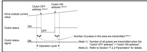
(e) When the "Clutch OFF" is set in the parameter "Error-time operation mode" of drive module and a major error occurs in the output module, the operating system software turns off the clutch.
