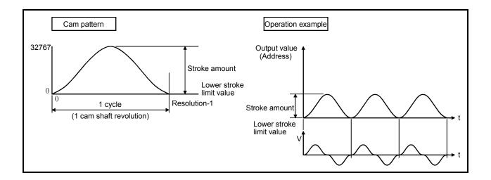
2) Feed cam mode ......With the lower stroke limit value (lower dead point) as the operation start position, positioning is executed by feeding one stroke amount per cycle in a fixed direction.
