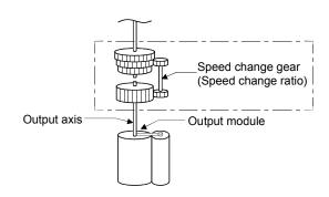
(2) When a speed change ratio changes, the acceleration/deceleration processing is executed by the smoothing time constant (t) set in the speed change gear parameters.
