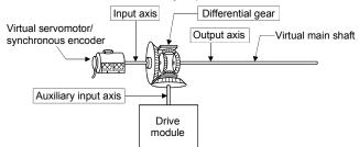
Set the different drive modules for virtual main shaft side and auxiliary input axis side.
