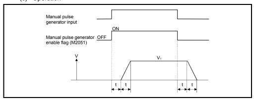
Output speed  $(V_1)$  [PLS/s] = (Number of input pulses/s) × (Manual pulse generator 1-pulse input magnification setting)
