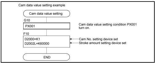
(Note): Example of the above Motion SFC program is started using the automatic start or PLC program.
