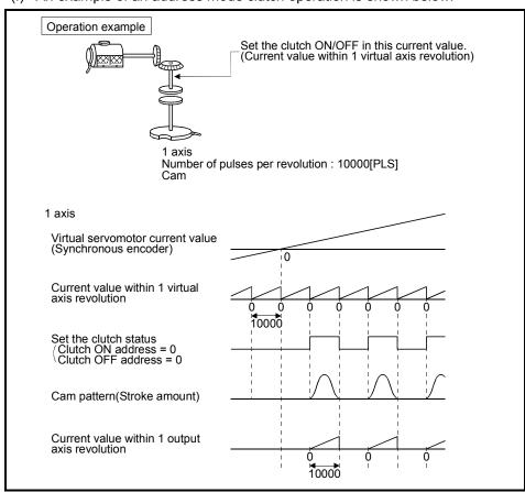
(f) An example of an address mode clutch operation is shown below.
