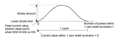
After the bottom dead point alignment of cam is completed at the system start-up, it must be turned on at the first real to virtual mode switching.
