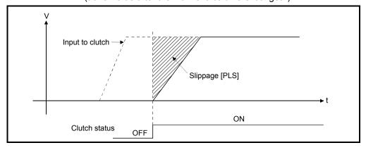
b) Execute the smoothing processing so that the slippage may become the shaded area by the linear acceleration/deceleration system at clutch ON/OFF. c) Since the slippage remains constant even if the drive module speed changes, the clutch ON/OFF position can be controlled without any influence from speed changes.
