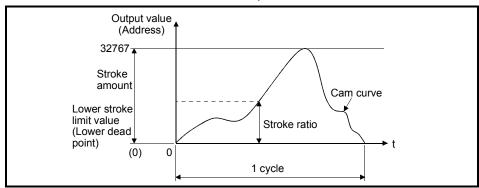
(b) The cam data table is automatically created by creating the cam curve using a peripheral device.
