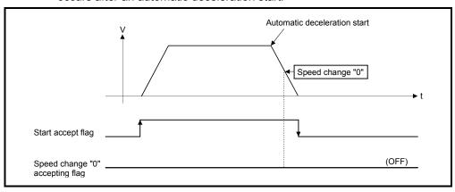
(d) Even if it is speed change "0" after the automatic deceleration start to the "command address", speed change "0" accepting flag turns on.
