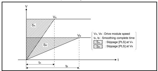
d) If input to clutch (travel value after the main shaft's differential gear) changes after smoothing completion, the smoothing processing is not executed and output directly.
