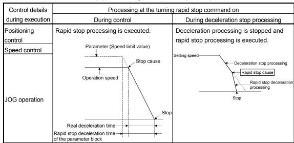
Table 4.2 Details of stop processing when the rapid stop command turns on
