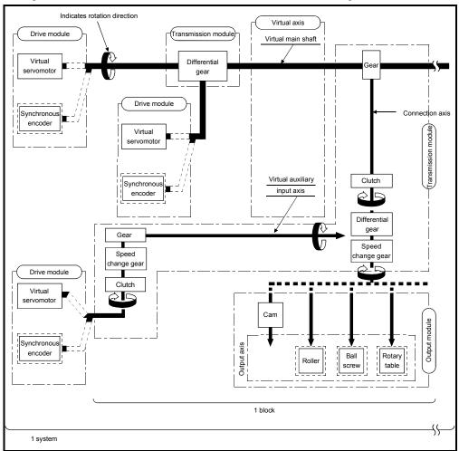
Fig. 5.1 Configuration of the Mechanical Module Connection
