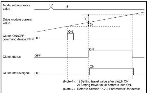
Fig. 7.5 Operation Timing for One-shot Mode
