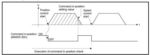
Fig. 6.1 Command in-position range
