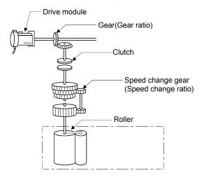
(b) When a clutch is used, the roller is controlled at clutch ON.
