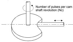
(b) The setting for the number of pulses per cam shaft revolution is not related to the travel value per pulse (fixed parameter setting).
