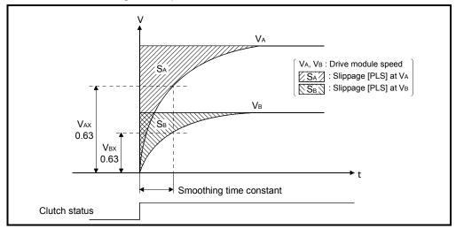
2) If input to clutch (travel value after the main shaft's differential gear) changes after smoothing completion, the smoothing processing is executed at that point.
