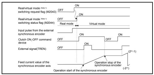
b) The control mode <sup>(Note-3)</sup> of a clutch is operation in the case of external input mode.
