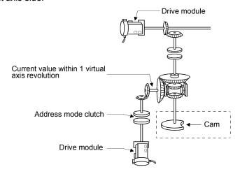
(a) By setting the current value within 1 virtual axis revolution of auxiliary input axis side, the current value within 1 virtual axis revolution is stored in the preset device.
