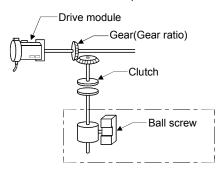
(b) When a clutch is used, the ball screw is controlled at clutch ON.
