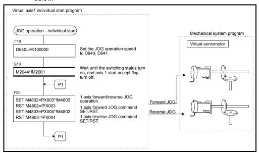
(Note): Example of the above Motion SFC program is started using the automatic start or PLC program.
