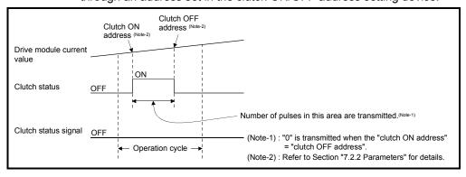
2) When the clutch status signal is ON and the current value passes through an address set in the clutch ON/OFF address setting device.
