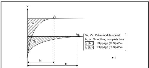
Input to clutch Travel value after the main shaft's differential gear Internal clutch status Slippage [PLS] Output to output axis Slippage [PLS] by the smoothing clutch for exponential function system Smoothing processing is not executed. Smoothing completion Smoothing completion Clutch status signal
