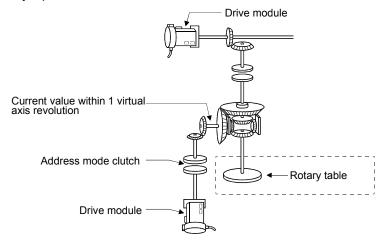
(a) By setting the current value within 1 virtual axis revolution of rotary table auxiliary input axis side for the current value within 1 virtual axis revolution is stored in the preset device.
