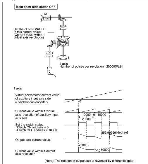
(f) An example of an address mode clutch operation is shown below.
