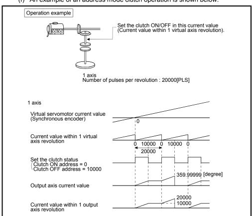
(f) An example of an address mode clutch operation is shown below.
