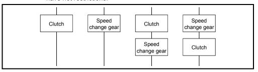
(b) Transmission module which can be connected at "C" (pattern 3) Only a clutch can be connected at "C".
