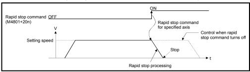
(b) The details of stop processing when the rapid stop command turns on are shown in Table 4.2.
