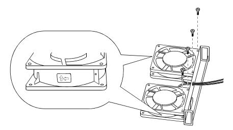
8) Reinstall the cooling fan to the power regeneration common converter unit in the reverse procedure.
