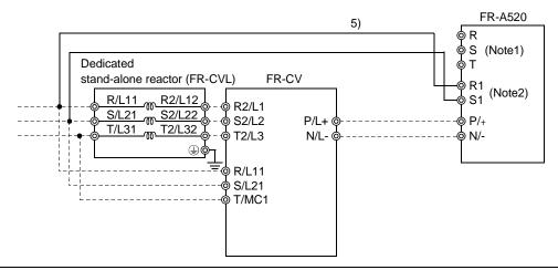
Note: 1. Never connect a power supply to the inverter terminals R, S, T. Accidental connection will damage the inverter and power regeneration common converter.
