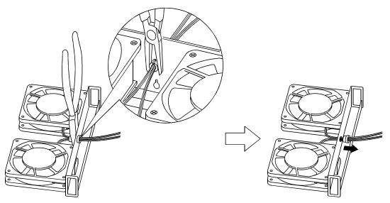
7) Remove the cooling fan from the cooling fan mounting fixture, and change the cooling fan. When reinstalling the cooling fan, take care so that the arrows given on the cooling fan point as shown below.
