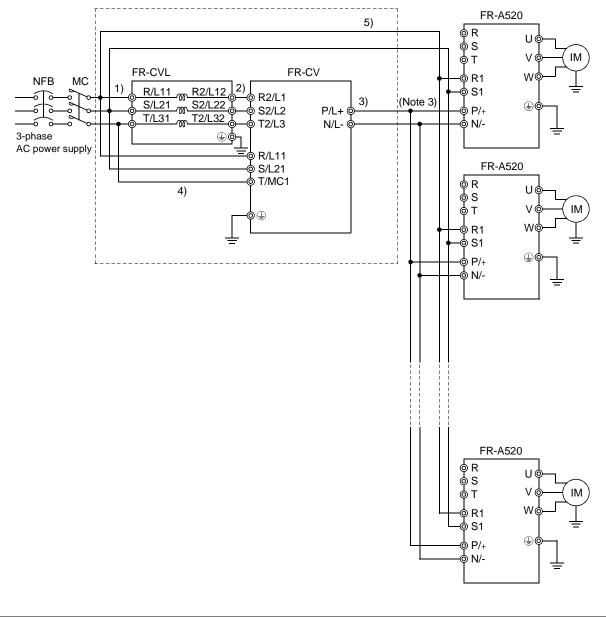
Note: 1. The cables used should be 75°C (167F°) copper cables. 2. Tighten the terminal screws to the specified torques. Undertightening can cause a short or misoperation.
