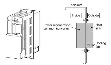
The FR-CV-37K, 55K and FR-CV-H37K, H55K can be used either as a heat sink outside mounting structure model or an enclosure inside installation structure model by changing its mounting foot position. It is shipped from the factory as a heat sink outside mounting structure model. Change the mounting foot position as shown below for installation.
