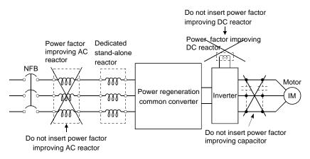
Note: A power factor improving capacitor or surge suppressor on the inverter's output may overheat or be damaged due to the harmonics of the inverter output. Also, when an overcurrent flows in the inverter, the overcurrent protection is activated, Hence, when the motor is driven by the inverter, do not install a capacitor or surge suppressor on the inverter's output. Do not use the power factor improving AC reactor (FR-BAL) since using it may degrade the power regeneration function.
