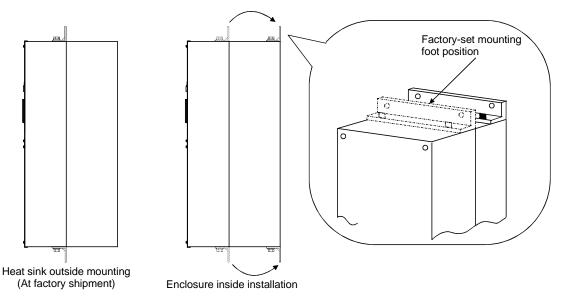
(2) Enclosure inside installation structure model (FR-CV-7.5K to 30K-AT, FR-CV-H7.5K to H30K-AT)
