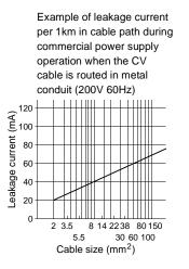
Leakage current example of 3-phase induction motor during commercial power supply operation (200V 60Hz)
